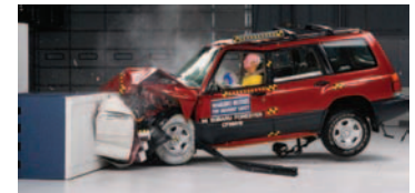
Figure 9.4 (Example 9.3) (a) This car's momentum changes as a result of its collision with the wall. (b) In a crash test, much of the car's initial kinetic energy is transformed into energy associated with the damage to the car.
