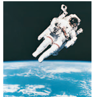
The force from a nitrogen-propelled hand-controlled device allows an astronaut to move about freely in space without restrictive tethers, using the thrust force from the expelled nitrogen.
