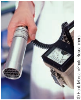
Figure 45.16 (a) Diagram of a Geiger counter. The voltage between the wire electrode and the metallic tube is usually approximately 1 000 V. (b) A scientist uses a Geiger counter to make a measurement.
