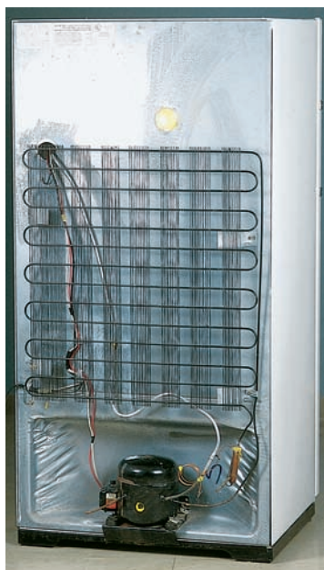
Figure 22.6 The coils on the back of a refrigerator transfer energy by heat to the air. Due to the input of energy by work, this amount of energy must be greater than the amount of energy removed from the contents of the refrigerator.
