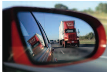
Figure 36.15 (Example 36.4) An approaching truck is seen in a convex mirror on the right side of an automobile. Because the image is reduced in size, the truck appears to be farther away than it actually is. Notice also that the image of the truck is in focus, but the frame of the mirror is not, which demonstrates that the image is not at the same location as the mirror surface.
