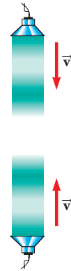
Figure 18.6 Two identical loudspeakers emit sound waves toward each other. When they overlap, identical waves traveling in opposite directions will combine to form standing waves.
