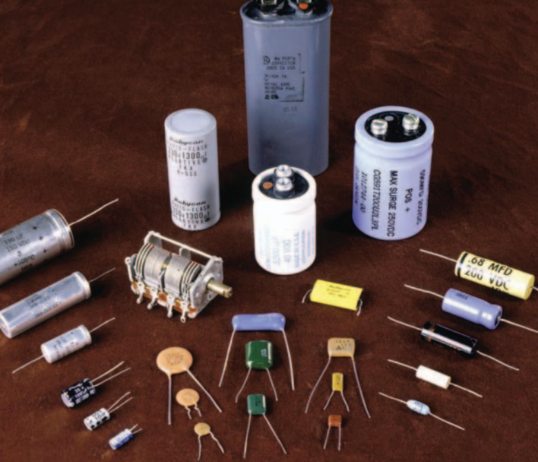
All these devices are capacitors, which store electric charge and energy. A capacitor is one type of circuit element that we can combine with others to make electric circuits. (Paul Silverman/Fundamental Photographs)
