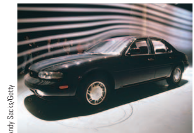
Figure 14.13 Laminar flow around an automobile in a test wind tunnel.
