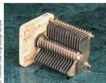
Figure 26.16 A variable capacitor. When one set of metal plates is rotated so as to lie between a fixed set of plates, the capacitance of the device changes.
