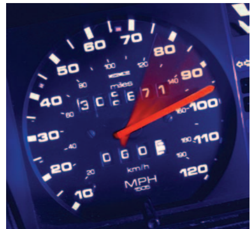
Figure 1.3 The speedometer of a vehicle that shows speeds in both miles per hour and kilometers per hour.
