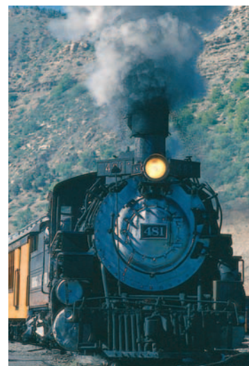
Figure 22.1 This steam-driven locomotive runs from Durango to Silverton, Colorado. It obtains its energy by burning wood or coal. The generated energy vaporizes water into steam, which powers the locomotive. (This locomotive must take on water from tanks located along the route to replace steam lost through the funnel.) Modern locomotives use diesel fuel instead of wood or coal. Whether old-fashioned or modern, such locomotives can be modeled as heat engines, which extract energy from a burning fuel and convert a fraction of it to mechanical energy.
