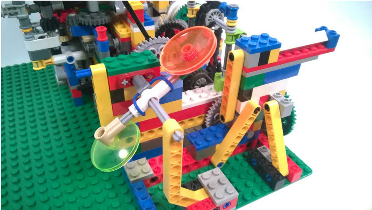
Fan Fly with single support, rubber band drive, and pendulum pivot cantilever supports.
