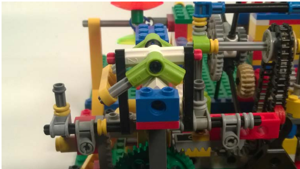
Knife-Edge pivot (light green) and 2 adjustable gravity "springs" controlling pallet resting position.
